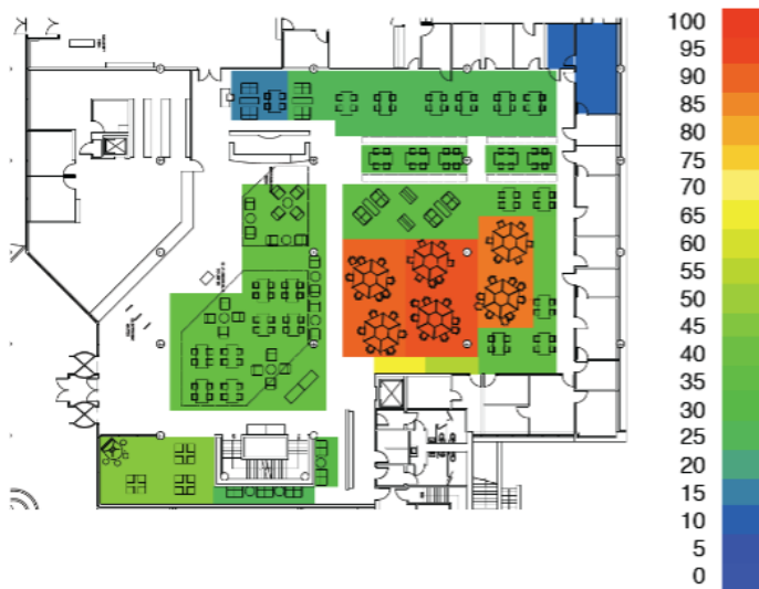
Figure 5: Prototype heat map for the entrance level of the Library. Relatively high occupancy areas are in red, relatively low occupancy areas in green/blue.
